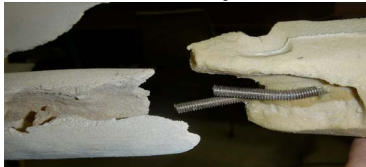
We used casting resin and stainless allthread to attach replicate jaw tip casts to the real bone.
