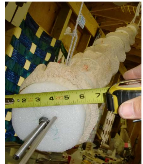
Stainless allthread and polycarbonate rod support tail section.
