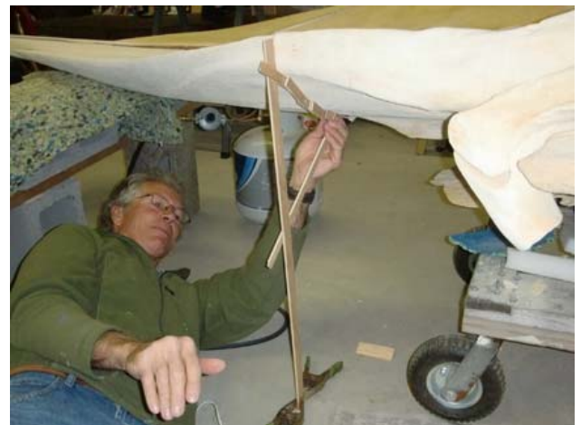
Stainless allthread and polycarbonate rod support tail section.
